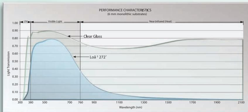
Transmitted and Exterior Appearance of Clear vs. LoE<sup>2</sup>-272 Glass.
