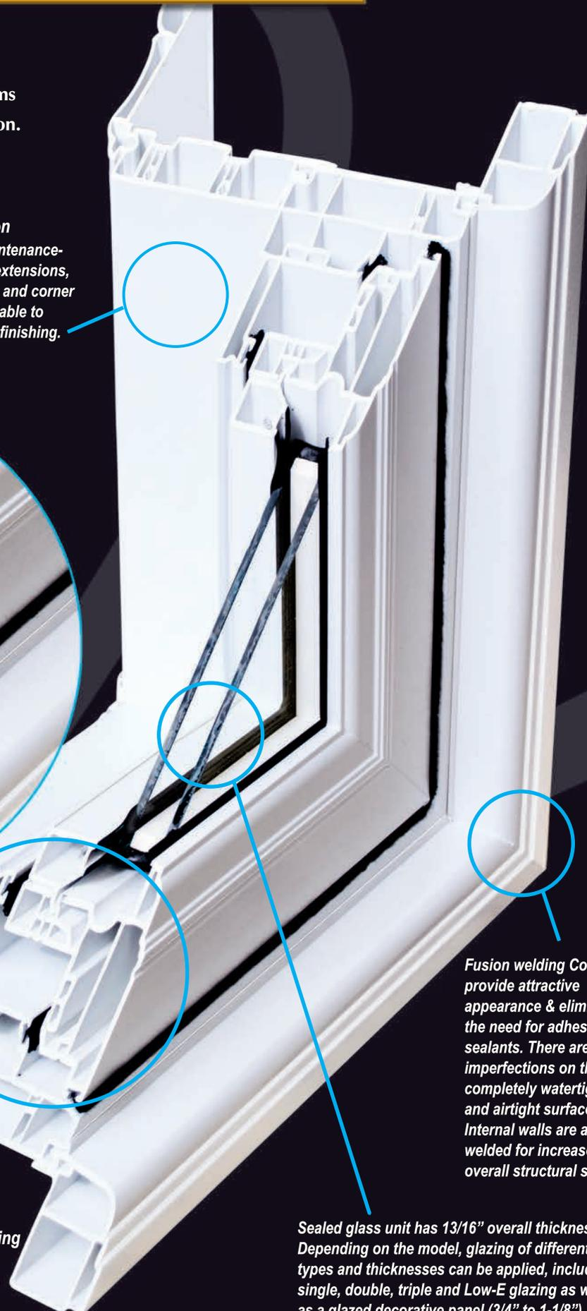
*Fusion welding Corners provide attractive appearance & eliminate the need for adhesive and sealants. There are no imperfections on the completely watertight and airtight surface. Internal walls are also welded for increased overall structural strength.*
